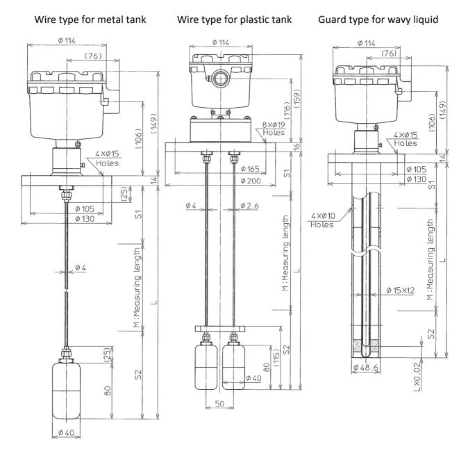
Note: The tensile strangth of wire for CG400BHF and CG400BDHF is 9.8 N Max.
